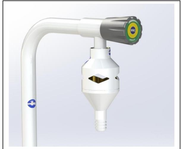
The product is designed specifically to protect the water supply against contamination from back siphonage within the laboratory environment. The nozzle must be permanently fitted to the outlet of the laboratory water tap with Loctite 648. The fitting of this nozzle will introduce the statutory air gap.
