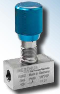
The RSD2 is a throttle valve which regulates the volume flow in the sensing/impulse line by means of a continuously adjustable cross-sectional reduction. The setting is made tool-free by means of a rotary knob and can be adjusted using a screw to be fixed. The throttle valve cannot be completely shut off, therefore a guaranteed minimum flow is ensured.
